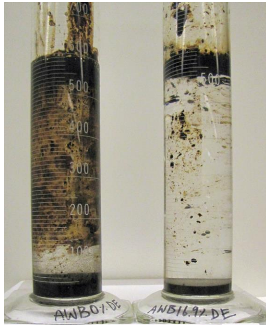
Figure 4-6. Mixture of the fresh (left) and W2 (right) fractions of AWB and 10 g/L diatomaceous earth sediment after 24 hours of settling. Note compact oil-sediment layer on bottom and oil layer on top. Photo: B.P. Hollebhone, Environment Canada
