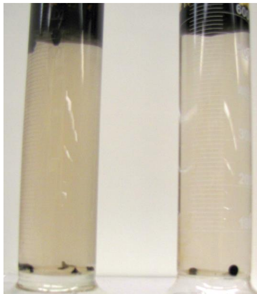
Figure 4-7. Mixture of the fresh (left) and W2 (right) fractions of CLB and 10 g/L sand sediment after 24 hours of settling. Photo: B.P. Hollebhone, Environment Canada
