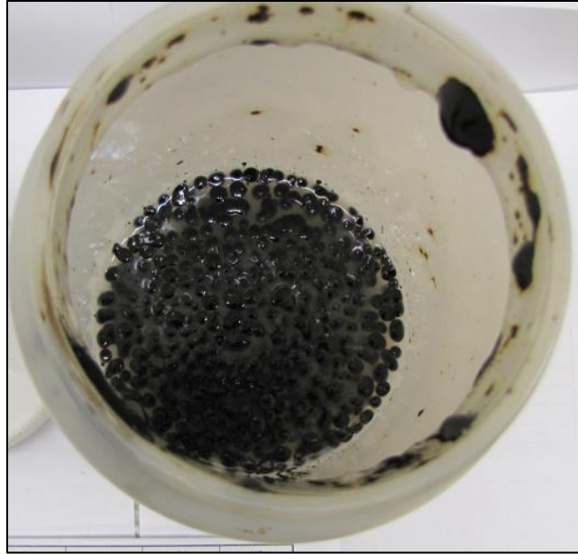
Figure 4-5. Mixture of the W3 fraction of AWB (25.34% mass loss) and 10 g/L kaolin sediment. Photo: B.P. Hollebhone, Environment Canada
