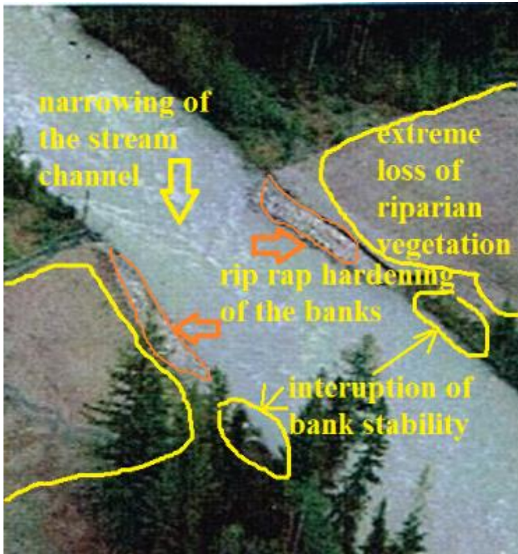
Figure 12 Extensive damage to the stream bank and riparian areas at a Trans Mountain pipeline crossing putatively in the Anchor Loop TMP project. For all intents-and-purposes, and from a fish-habitat perspective, this stream crossing can be viewed as a “biological scorched-earth zone”. Figure adapted (notations on photo, SRES additions) from May 19/20, 2015 TMP information meetings (presentation powerpoint by Calum Bonnigton).
