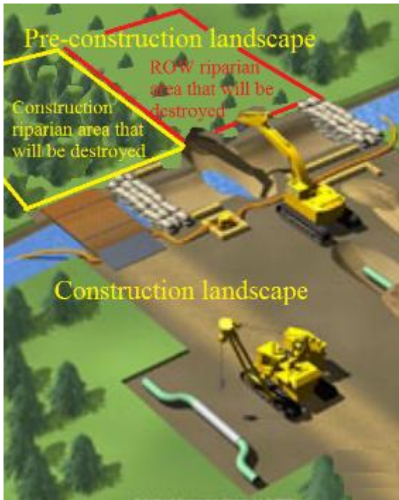
Figure 26 Pipeline construction across a stream using trenching methodology as proposed by Trans Mountain Expansion Project for most of its stream crossings.
