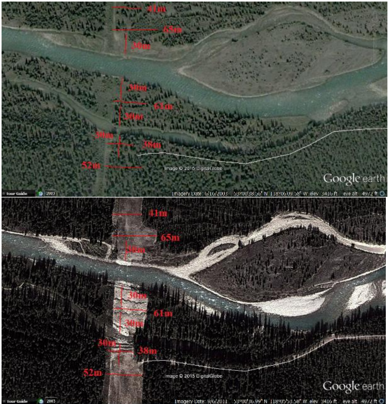
Figure 14 Extreme and extraordinarily unmitigated fish-habitat damage in the riparian areas of Snaring River and side channels caused by the Anchor Loop construction. Top photo shows Google Earth air photo taken June 16, 2003, prior to the Anchor Loop construction; bottom photo shows Google Earth air photo taken September 6, 2011 three years after the end of construction. Note the extensive amount of live large-woody vegetation within the 30 m riparian zone, in 2003, that was destroyed between 2004-2008. Note, as well, the profoundly impacted impacts to ephemeral channels within the island. Finally, note, that in many instances the vegetation removal far-and-away exceeds the 45 m corridor widths indicated by TMP at the public meetings and in the TMEP documents. Distances determined from Google Earth app.
